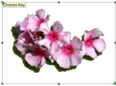
In this example, the background color was sampled using Apple's Colors palette. The Tolerance slider was given a setting of 20% so that all the green was made transparent.
